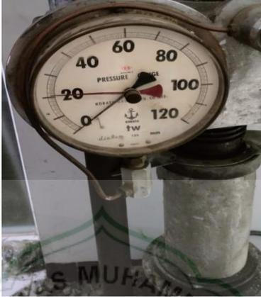
A close-up photograph of a circular pressure gauge with a white face and black markings. The scale ranges from 0 to 120 with major increments every 20 units. The needle is positioned at approximately 21. The gauge is mounted on a metal stand and is connected to a concrete test specimen.   | 21          |
