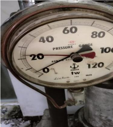
A close-up photograph of a circular pressure gauge with a white face and black markings. The scale ranges from 0 to 120 with major increments every 20 units. The needle is positioned at approximately 23. The gauge is mounted on a metal stand and is connected to a concrete test specimen. | 23          |
