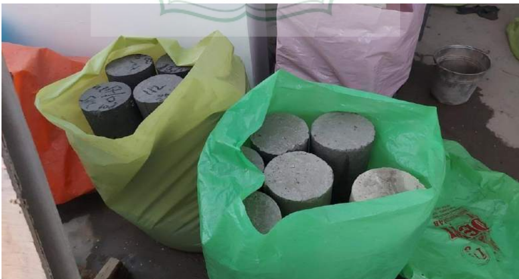
Gambar 3.25 Perawatan/perendaman Beton Silinder
