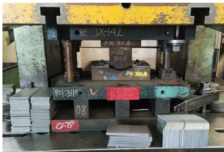
Figure 2: Construction of conventional die
