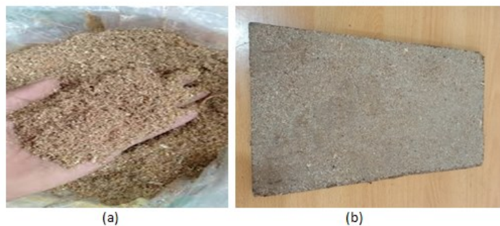
Figure 2. Insulation materials (a) teak wood sawdust and (b) compacted board
