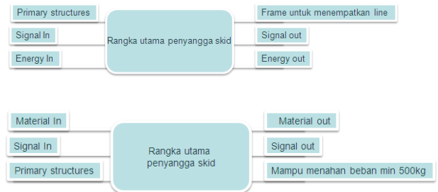
Gambar 2. Fungsi Primary Structure.
