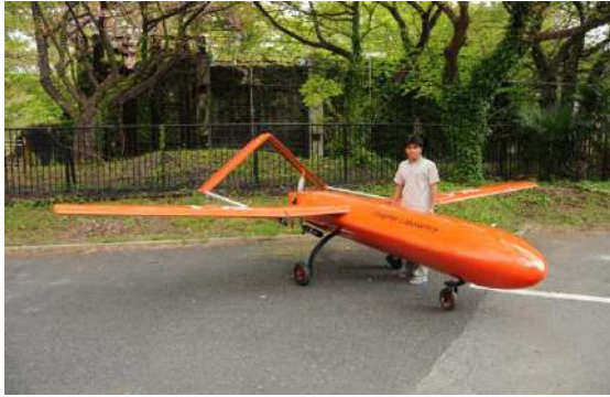
Figure 2. Josaphat experimental unman aerial vehicle (JX-1 UAV); a) UAV configuration, b) Photograph of the UAV
