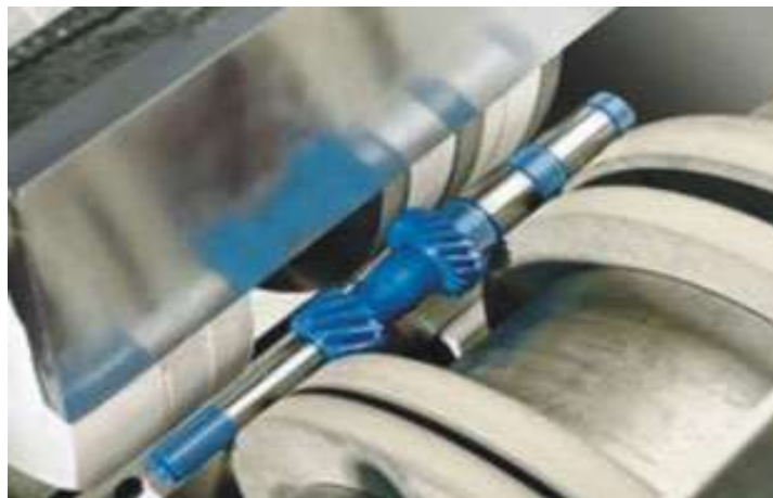
Gambar 6.5. Proses gerinda centerless
