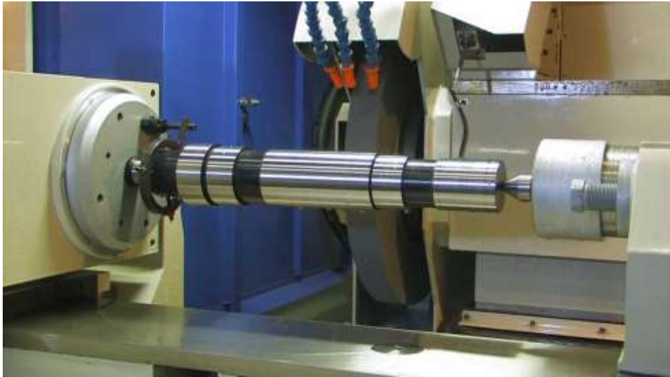
Gambar 6.2. Proses gerinda silindris
