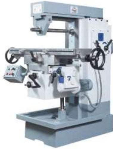
**Gambar 4.4.** Mesin Frais Horizontal
