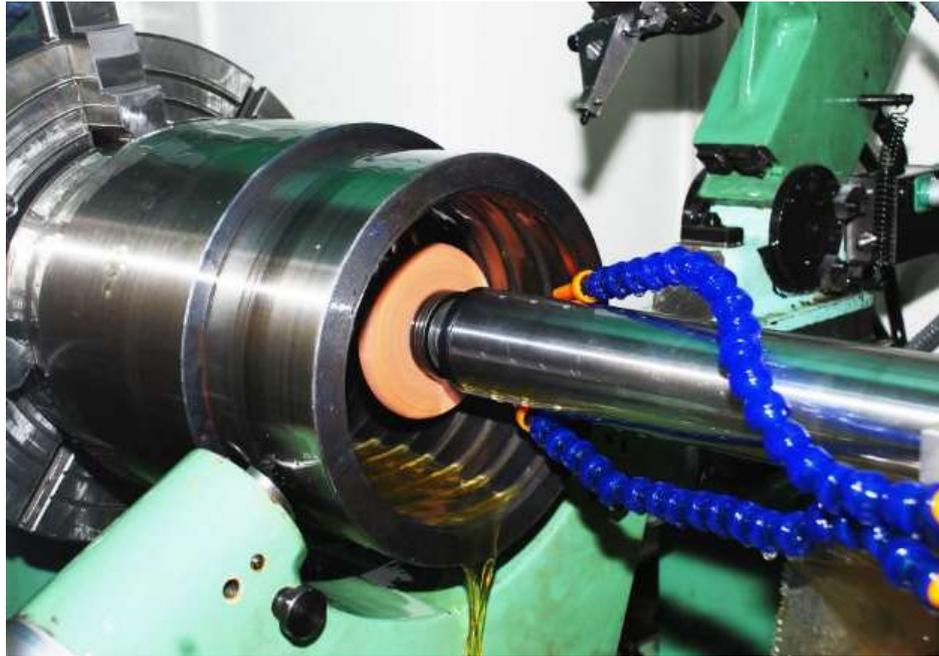
**Gambar 6.4.** Proses gerinda dalam/ internal
