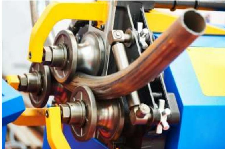
**Gambar 9.9.** Skema proses *Roll-Bending*
