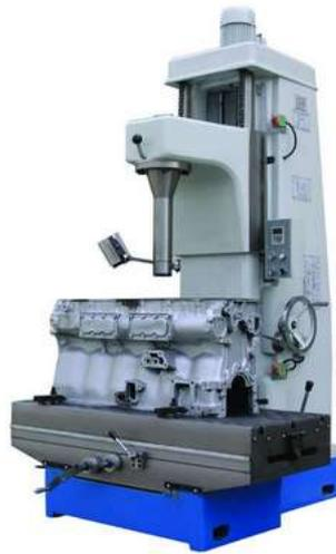
**Gambar 2.6.** Mesin Boring
