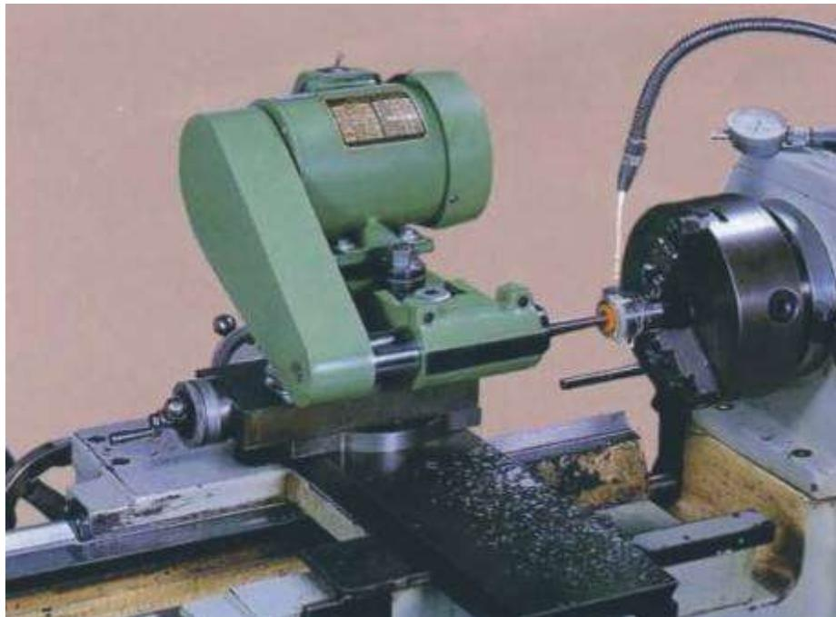
**Gambar 6.3.** Mesin gerinda dalam/ internal
