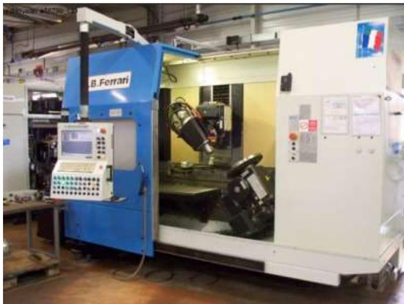
**Gambar 7.3.** Mesin CNC 5 Axis
