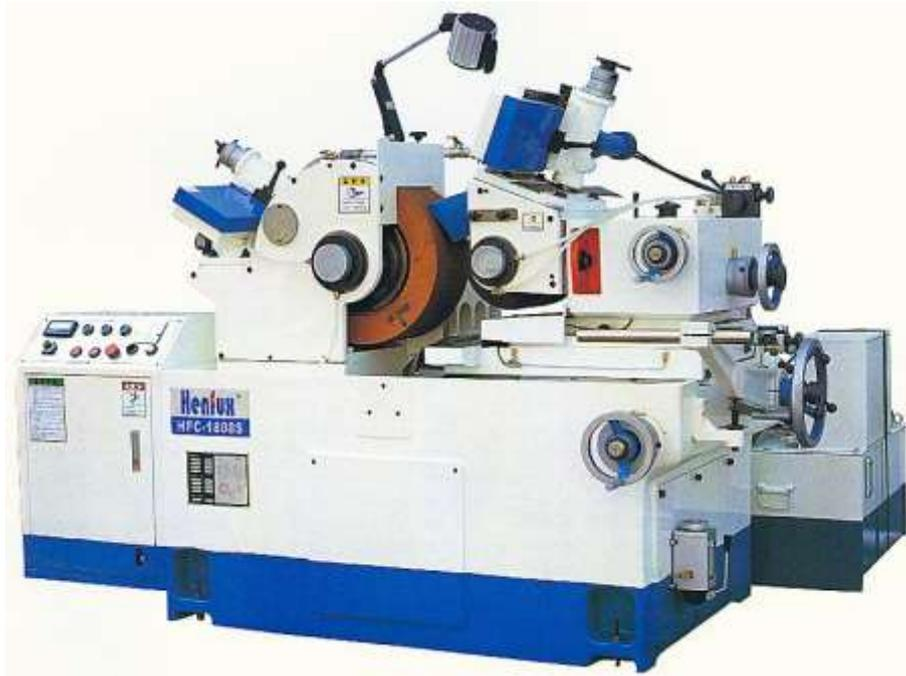
**Gambar 6.6.** Mesin gerinda *centerless*
