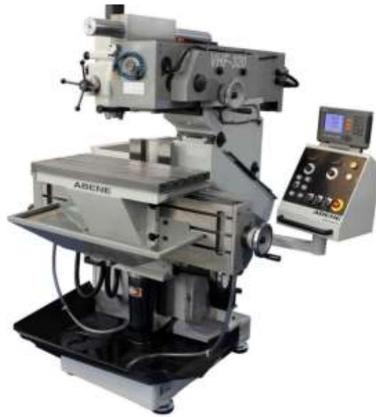
**Gambar 4.6.** Mesin NC Mills/ Frais
