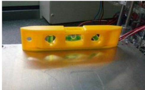
Fig. 3. Levelling method using sprit level tool
