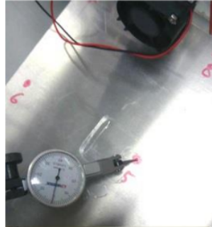
Fig. 4. Levelling method using dial indicator gauge
