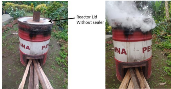
Figure 4. Thick smoke produced by kiln without sealer
