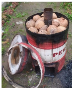
Figure 3. The coconut shells were arranged neatly to fill up the kiln.
