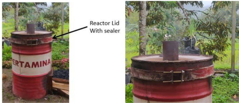
Figure 5. Very thin smoke appears at the kiln with sealer
