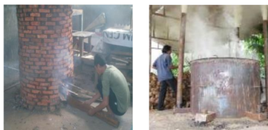
92 Figure 1. The carbonization process created a lot of smoke that pollutes the air
