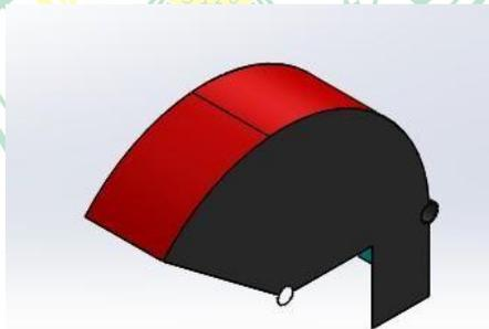
**Gambar 3. 10** Desain fender roda
