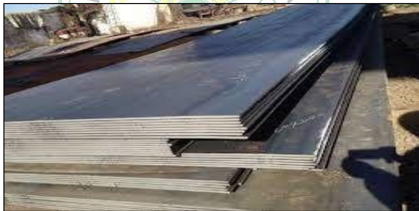
Gambar 2.3 Baja lembaran ASTM A36 tebal 1,2 mm
