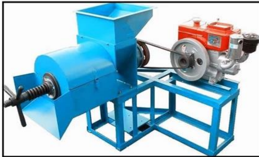
Gambar 2.10 Alat pres screw gambir
