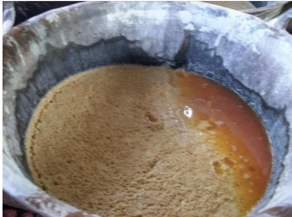
Gambar 2.5 Proses pengendapan getah gambir
