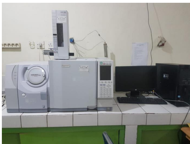
101 102 Figure 1. Gas Chromatography GC GC-MS Shimadzu QP 2010S (Shimadzu Corp, Kyoto, Japan).
