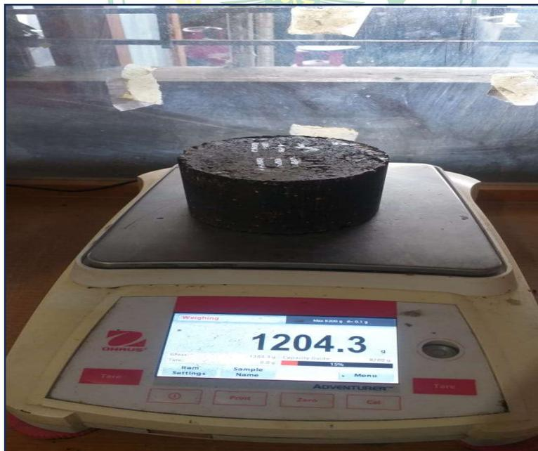
Gambar 4. Penimbangan Agregat Campuran AKAP
