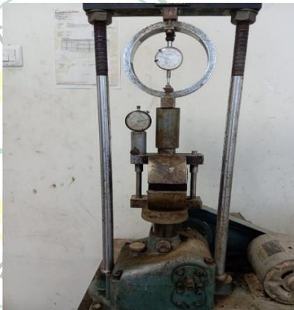
Gambar 3.9 Alat *Marshall Test*
