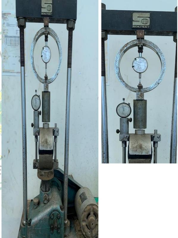
Two photographs of a Marshall Test Machine. The left image shows the machine from a side view, highlighting the vertical frame, the upper and lower anvils, and the central loading mechanism. The right image shows the machine from a front view, focusing on the circular dial gauge used to measure the deformation of the specimen. The machine is labeled 'SOLTESY' at the top. A watermark for 'UNIVERSITAS M SUMATE' is visible on the left side of the images. |
