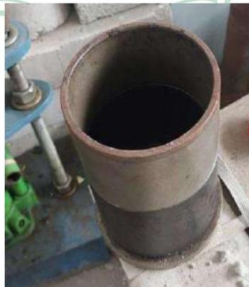
Gambar 3.8 Cetakan Benda Uji (Mold *Marshall* Test)
