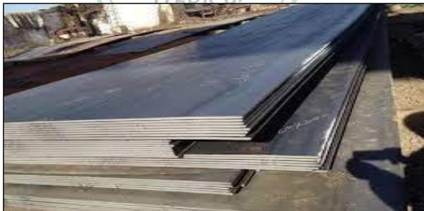
**Gambar 2.13** Baja lembaran ASTM A36 tebal 3 mm[15]
