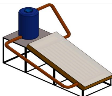
Gambar 2. Alat Solar Water Heater
