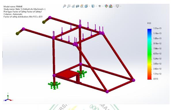
For the distribution of the minimum safety factor value that occurs in the frame of the corn thresher machine, it is shown in the figure above and the value obtained is 0.51.
