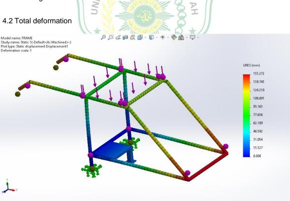
Based on the figure above, the total deformation simulation results on the frame show that the largest displacement that occurs is 155.272 mm while the smallest displacement value is 15.527 mm.
