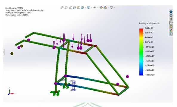
From the results of the stress analysis simulation by giving a loading of 10,000N (1000Kg) on the structure, the bending stress results were obtained. In the figure above, the largest von misses stress value is 940.6 N/mm2, while the smallest upper bound axial and bending stress value is 15.1 N/mm2.
