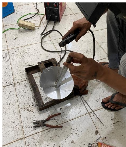
Gambar 3.17. Proses pengelasan screw
