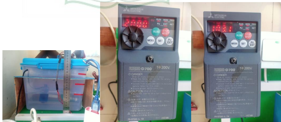
Gambar 4.9.. Kondisi volume reservoir hamper habis, Frekuensi 20 Hz, Tegangan 101.1 Volt, VSD mode low Speed
