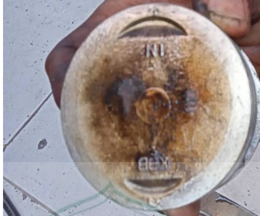
Gambar 3.12 Piston tiger 64,5 mm
