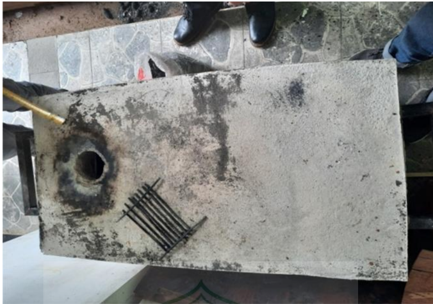
Gambar .3.4 Tungku re-heating lubang output diameter 100 mm
