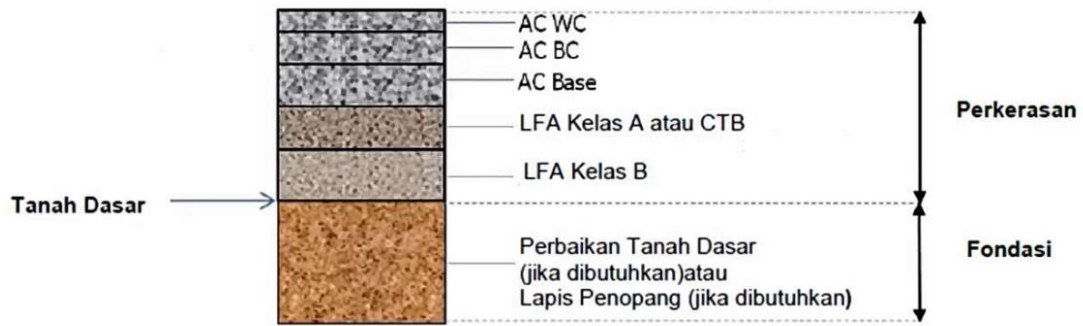
Gambar 4.2 Lapis Perkerasan Sumber : MDP No. 02/M/BM/2017
