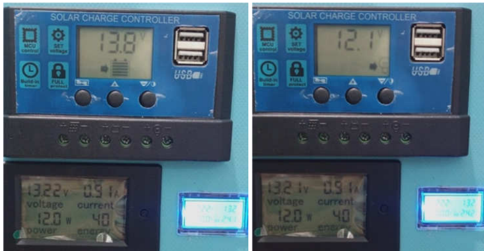
Gambar 3.35. Pengujian solar charger controller
