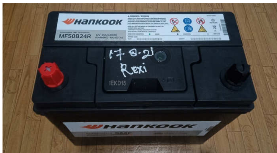
Gambar 3.19. Akumulator 12V 45 Ah
