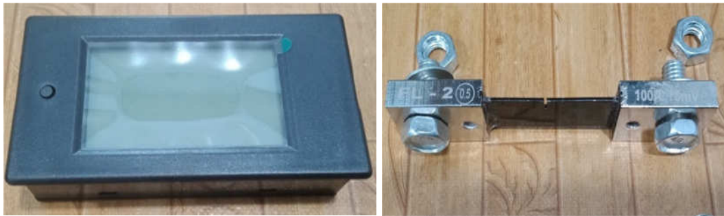
Gambar 3.21. KWh DC ammeter 100A 100 V dan Shunt 100 A 75mV
