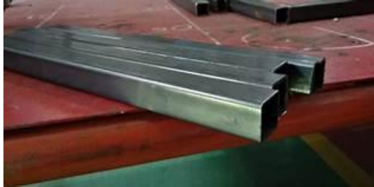
Gambar 3.8. Hollow structural section (HSS)
